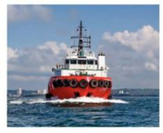
The 'Green Belait' was constructed under survey to ABS and features the notations + A1, OSR-S1, Offshore Support Vessel, + AMS, and CRC
