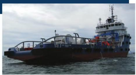
Designed by Conan Wu & Associates and built by Malaysia's Sarawak Slipways for Offshore Marine Services, the steel OSV 'OMS Resolution' was constructed under survey to ABS.
